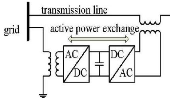
Fig.1a Simplified representation of a UPFC
