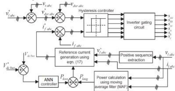
Fig. 3. Control block diagram for UPQC.
