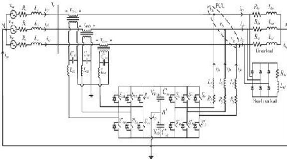
Fig. 1. Equivalent circuit of neutral-clamped VSI topology-based UPQC.
