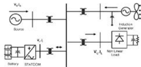
Fig. 3. Grid connected system for power quality improvement.
