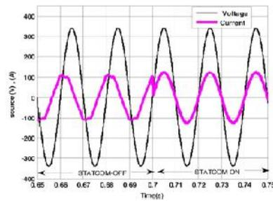
Fig. 5. Fig. 9. Supply Voltage and Current at PCC.
