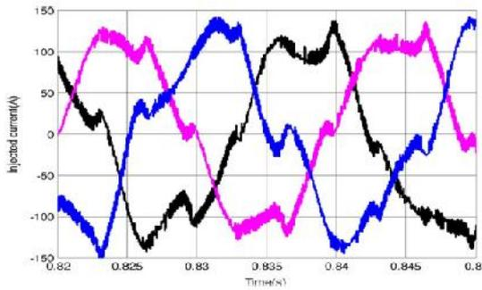
Three phase injected inverter Current.
