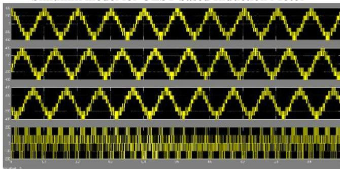
Three Phase Voltages  $V_{ab}, V_{bc}, V_{ca}$  & phase to neutral voltage  $V_{an}$
