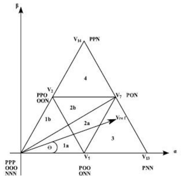
Fig. 4. Space vector diagram of sector 1 for a three-level inverter.
