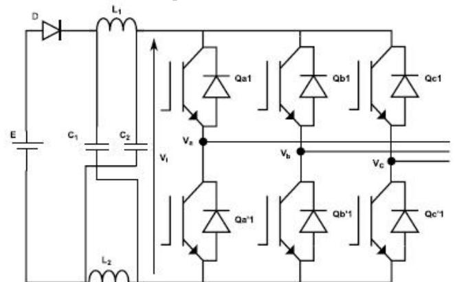
Fig. 1. Topology of two-level Z-source inverter.
