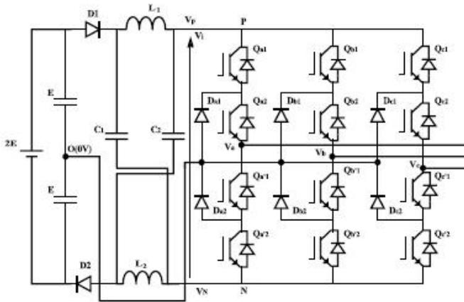
Fig. 2. Topology of an REC Z-source NPC inverter.
