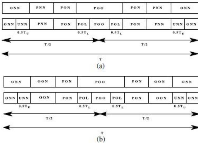
Fig. 5. Modulation of traditional NPC and Z-source NPC when the reference vector is in (a) triangle 3 and (b) triangle 2a on the three-level vector diagram shown in Fig. 4.
