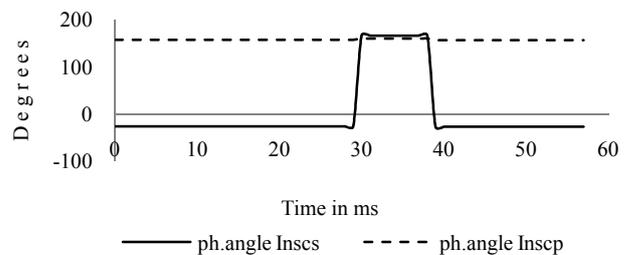
Fig. 6. Phase shift between Inscs to Inscp when 1% turns are shorted
