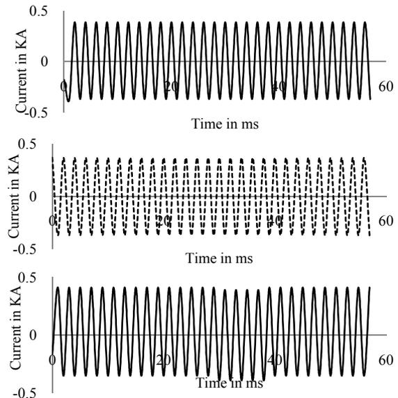
Fig. 2. Three Phase currents on primary side when 1% of turns are shorted in phase C.
