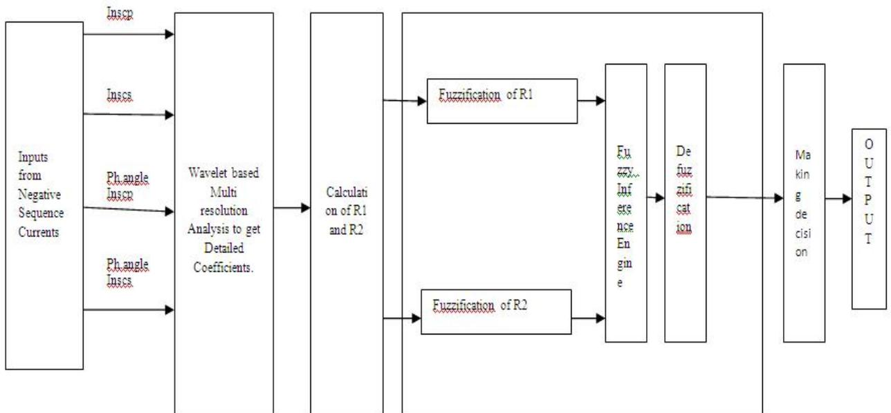
Fig. 12. Block diagram of the proposed algorithm
