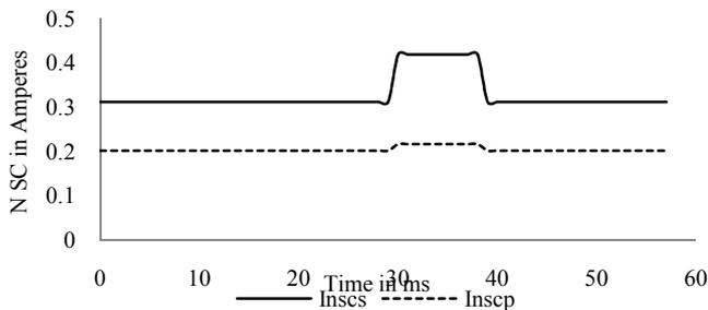
Fig. 4. Negative sequence current magnitudes on secondary and primary for 1% shorted turns on secondary in phase C.
