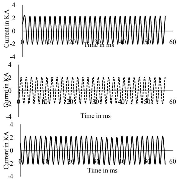
Fig. 3. Three Phase currents on secondary side when 1% of turns are shorted in phase C.
