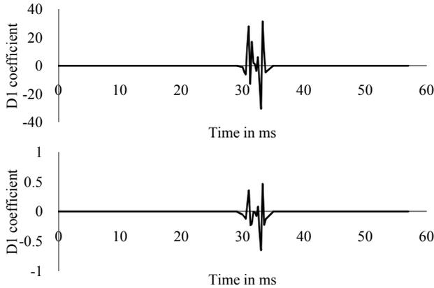
Fig. 7. d1 coefficient of phase varying signals when 1% turns are shorted.
