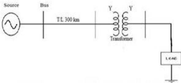
Fig. 1. One line diagram of power system model.
