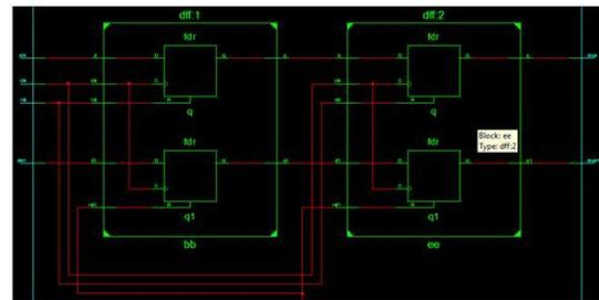
**Fig. 9 RTL view of SISO using MBFF**
