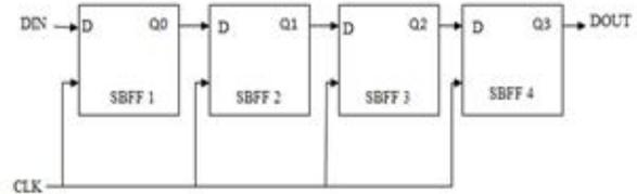
Fig. 5 SISO shift-register using single-bit flip-flop
