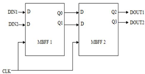
**Fig. 8 SISO shift-register using multi-bit flip-flops**
