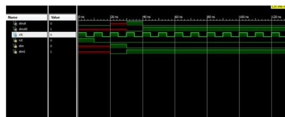
**Fig. 10 Output waveform of SISO using MBFF**
