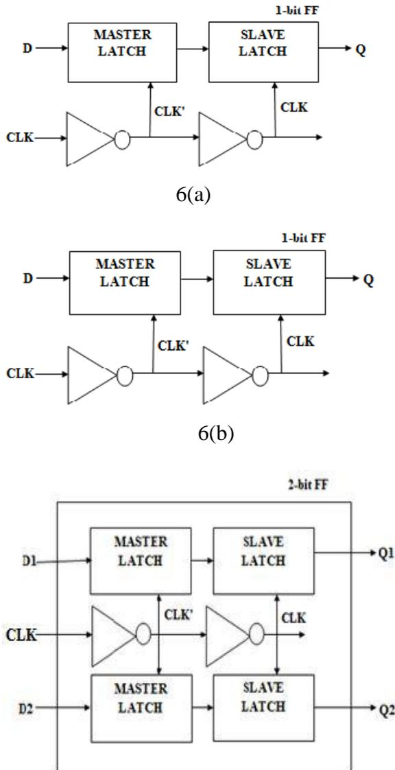
Fig. 6 Example of merging two 1-bit flip-flops into one 2-bit flip-flop.
