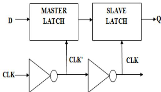
Fig. 4 Single-bit flip-flop
