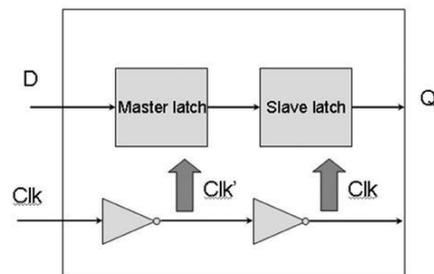
**Fig. 1 Single bit flip-flop**
