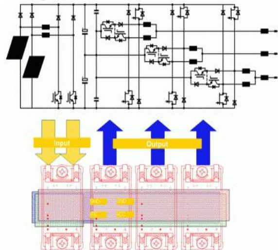
Fig. 1. PV modules and the multi-level PV inverter.
