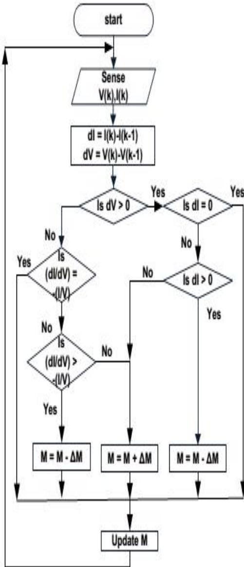
Fig. 4. Flow chart of Incremental Conductance MPPT
