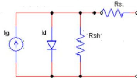
Fig.3. Equivalent circuit of solar cell
