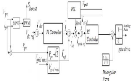
Fig.6 Control system for grid interfacing of PV system
