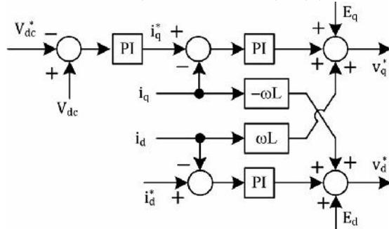
Fig. 2. Voltage controller for  $V_{dc}$ .
