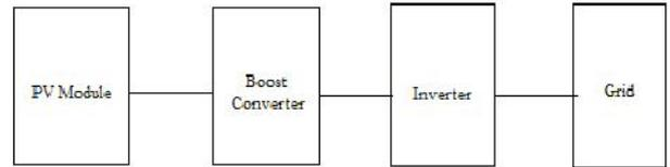
Fig.5. Block schematic of grid connected PV system
