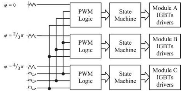
Fig.7. Modulation diagram for the seven-level inverter
