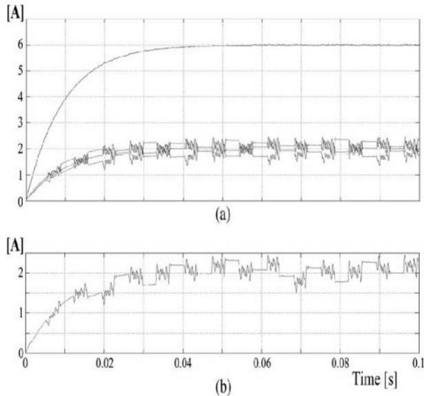
Fig. 12. Inductor current balance. (a) Inductor current. (b) Sharing inductor current detail.
