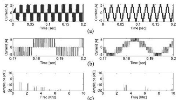
Fig.6. Comparison of three-level CSI and the seven-level MCSI. (a) Output current waveform. (b) Output current waveform detail. (c) Output current spectra.
