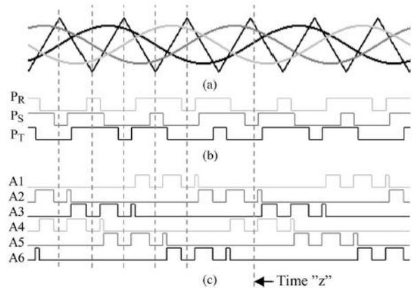
Fig.3. SPWM modulation
