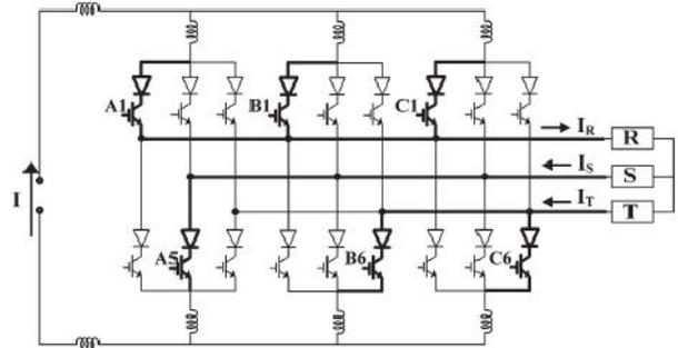
Fig.2. Current flow for a given switch configuration
