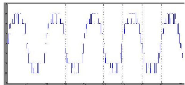
Fig. 9 seven level output
