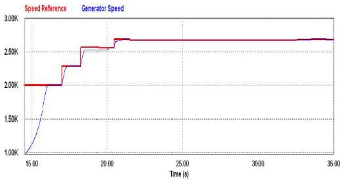
Figure 14 : Wind MPPT – Generator speed and reference speed signal (SEPIC operation)
