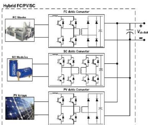
Fig. 2. Proposed structure of the hybrid FC/PV/SC power source.
