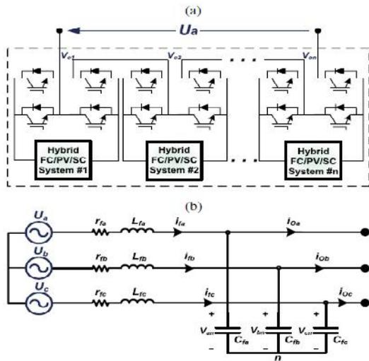
Fig. 1. (a) One-phase structure of a CHB multilevel inverter and (b) circuit diagram of a three-phase, three-wire DG unit.
