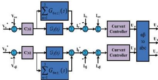
Fig. 3. Block diagram of the proposed multi-PR controller.
