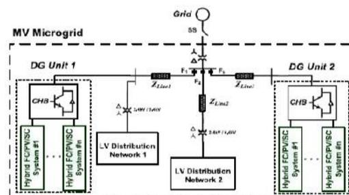
Fig. 4. Single-line diagram of MV microgrid consisting of two DG units.
