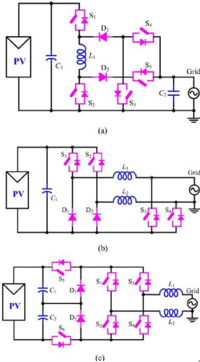
Fig. 3. Other transformerless inverter topologies: (a) Karschny inverter [19];(b) paralleled-buck inverter [20]; (c) H6 inverter with capacitor voltage divider [21]
