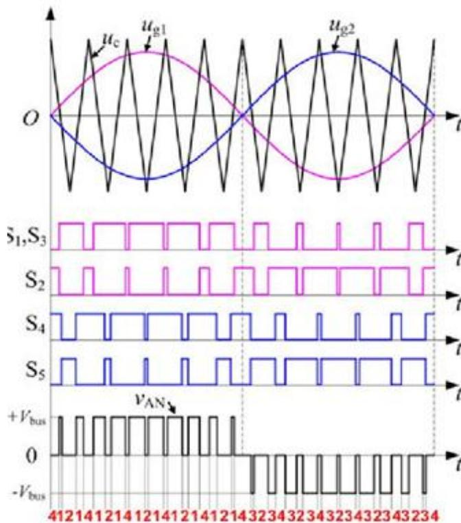
Fig. 6. Double SPWM for the proposed topology
