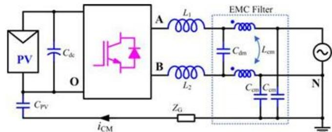
Fig. 1. CM current path for the transformerless PV inverter
