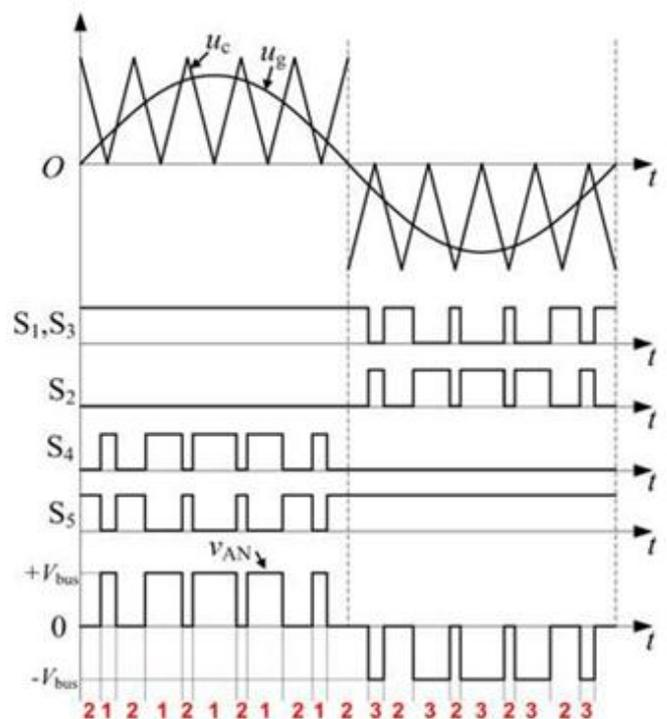
Fig. 5. Unipolar SPWM for the proposed topology.
