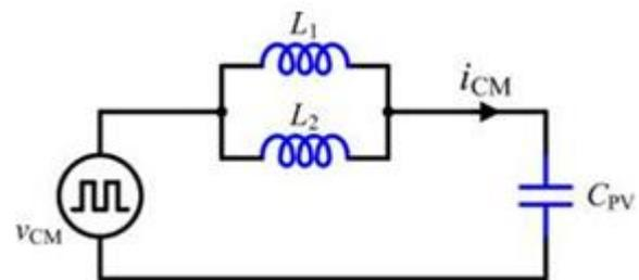
Fig. 2. Equivalent circuit for the CM current path combine cells of different voltage ratings [5], [6], different topologies], or even combine switch converters.
