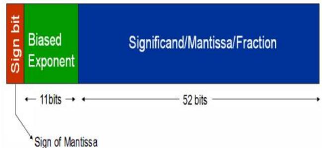
Figure1. IEEE 754 Double Precision Floating Point Format. The double precision floating point multiplier presented here is based on IEEE-754 binary floating standard. We have designed a high speed double precision floating point multiplier using Verilog language. It operates at a very high frequency of 414.714 MFlops and occupies 648 slices. It handles the overflow, underflow cases and rounding mode.
