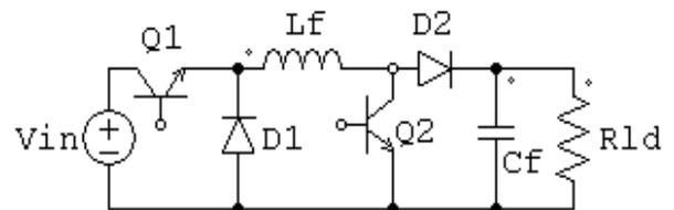
Fig.1. Two switch buck boost converter
