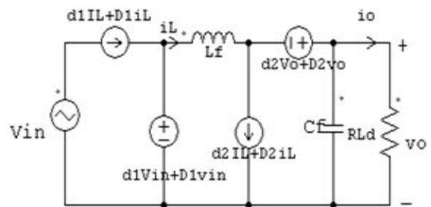
Fig.3(c) Small signal model
