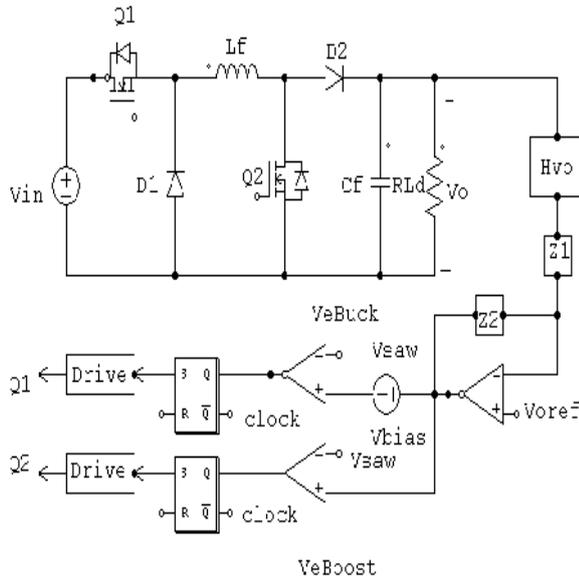
Fig.2. TSSB converter under the two mode control scheme
