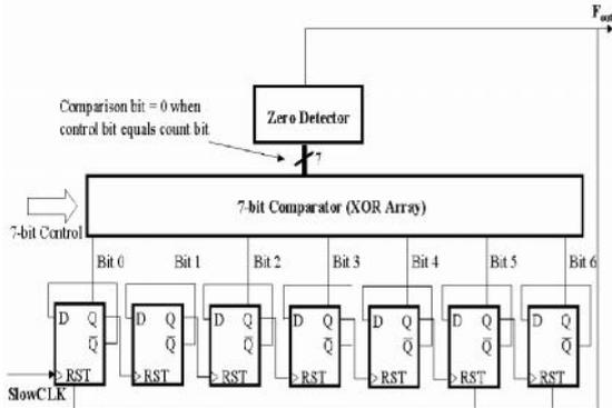
Fig.6. Block Diagram Of A 7-Bit Program Counter
