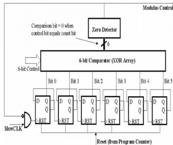
Fig.4. Asynchronous 6-bit S-counter.
