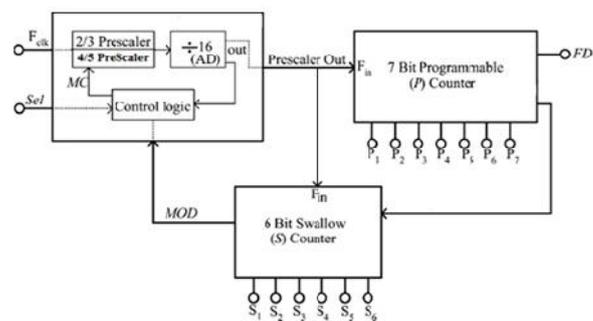
Fig.1. Proposed dynamic logic multiband flexible divider.
