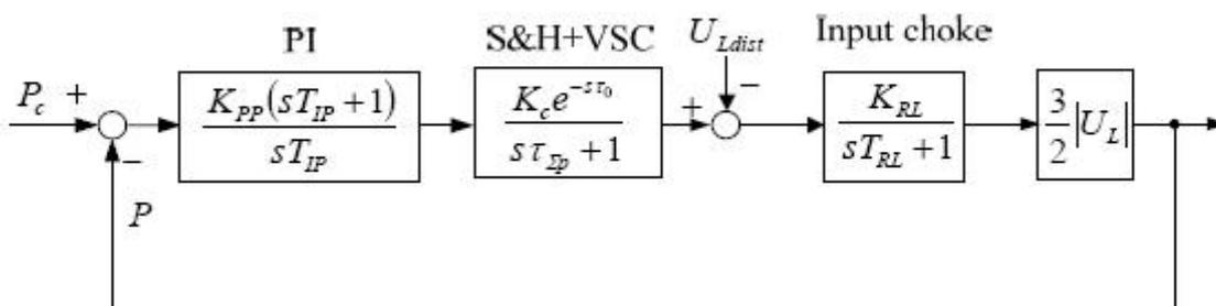
Fig. 4.6. Modified block diagram of Fig. 4.5
