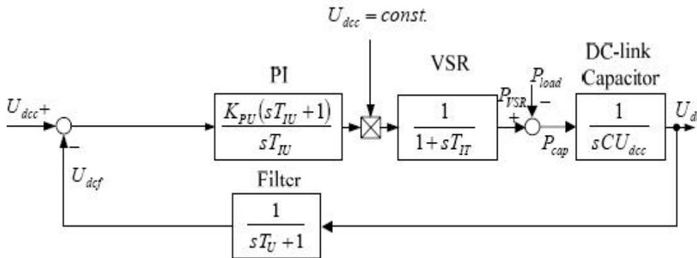
Fig. 4.7. Block diagram for a simplified DC-link voltage control loop
