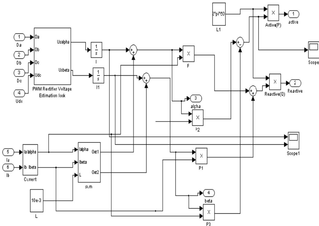
Fig 6.4. Simulink Inner block for active and reactive power estimation
