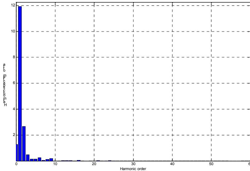
Fig.7.3. Total harmonic Distortion of Input Current of DPC with active filtering function
