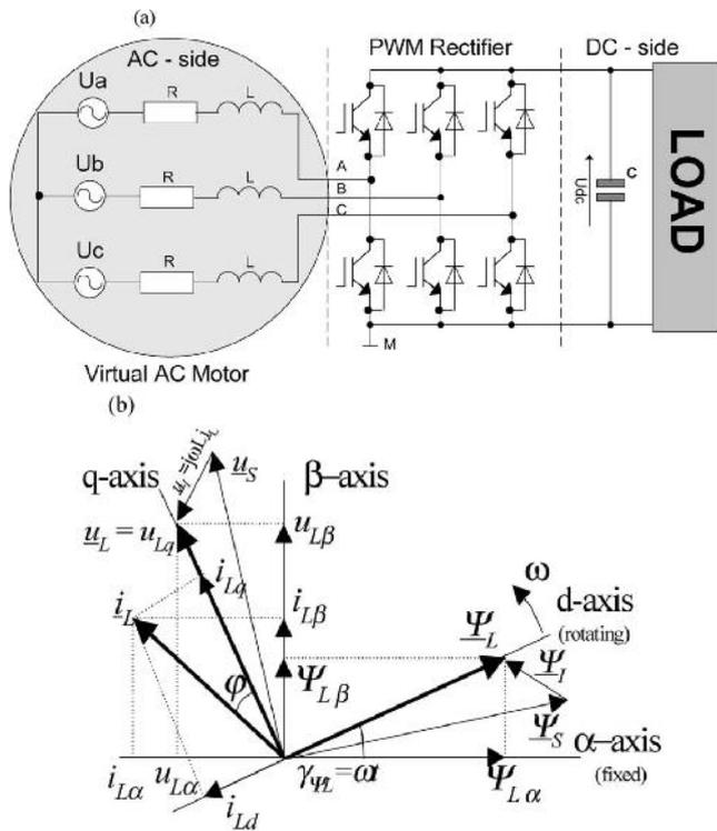
Fig. 4.2. (a) Three-phase PWM rectifier system with ac side presented as virtual ac motor.
