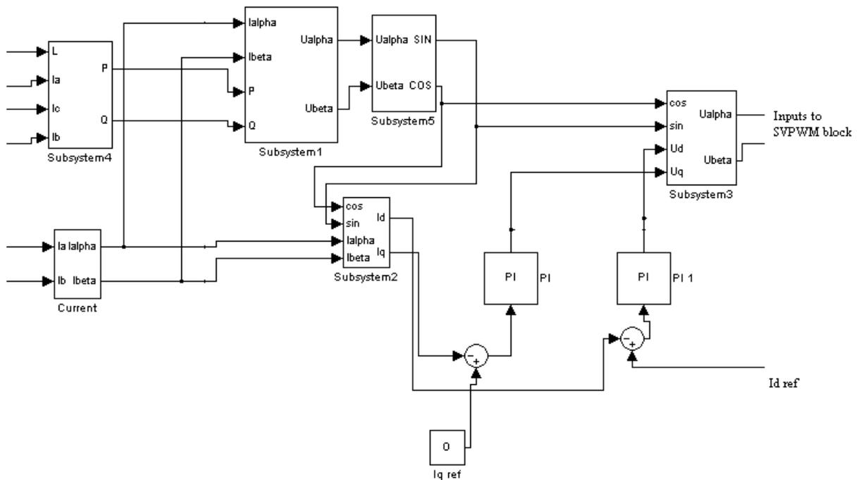
Fig 6.1. Simulink block for Voltage Oriented Control (VOC)
