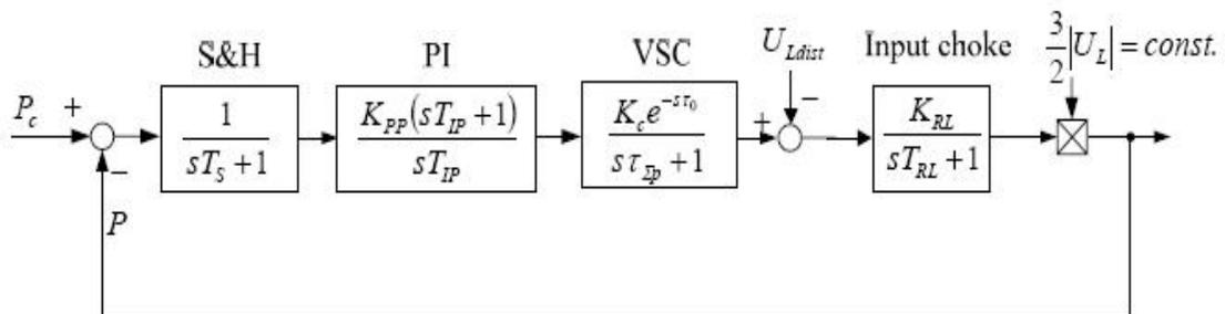
Fig. 4.5. Block diagram for a simplified active power control loop in the synchronous rotating reference frame
