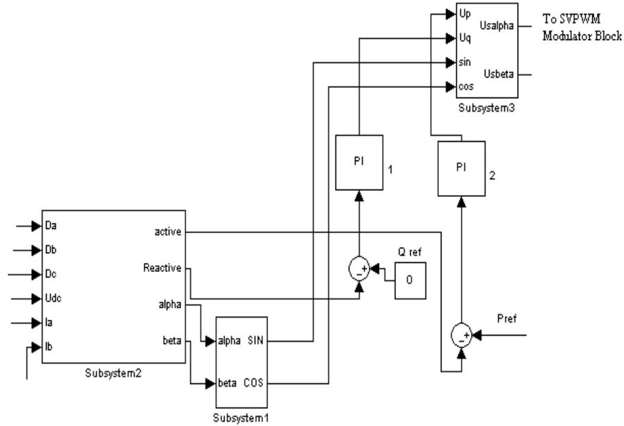
Fig 6.3. Simulink block for Direct Power Control (*DPC*)
