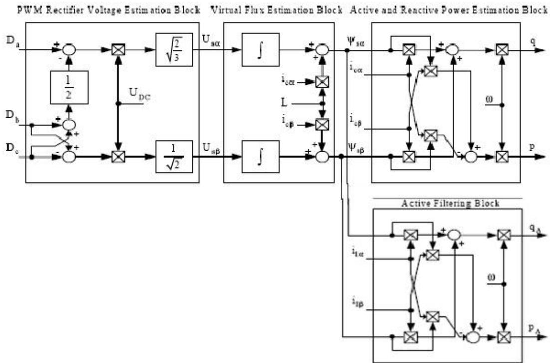
Fig. 6.6. Simulink block diagram for Power Estimators
