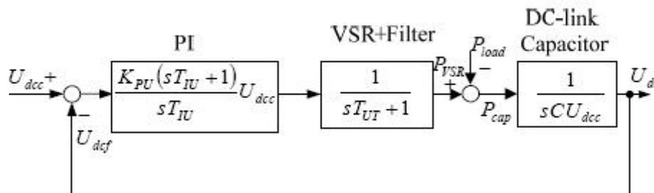
Fig. 4.8. Modified block diagram of Fig. 4.7
