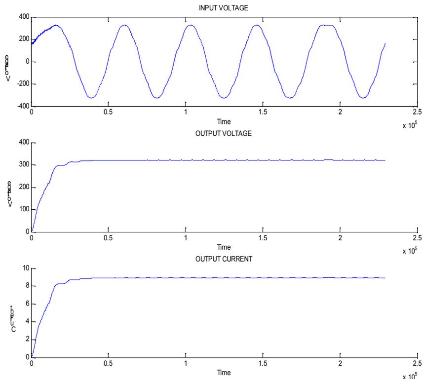
Fig 6.7(a). Waveforms of i) Input Voltage ii) Output Voltage iii) Output Current
