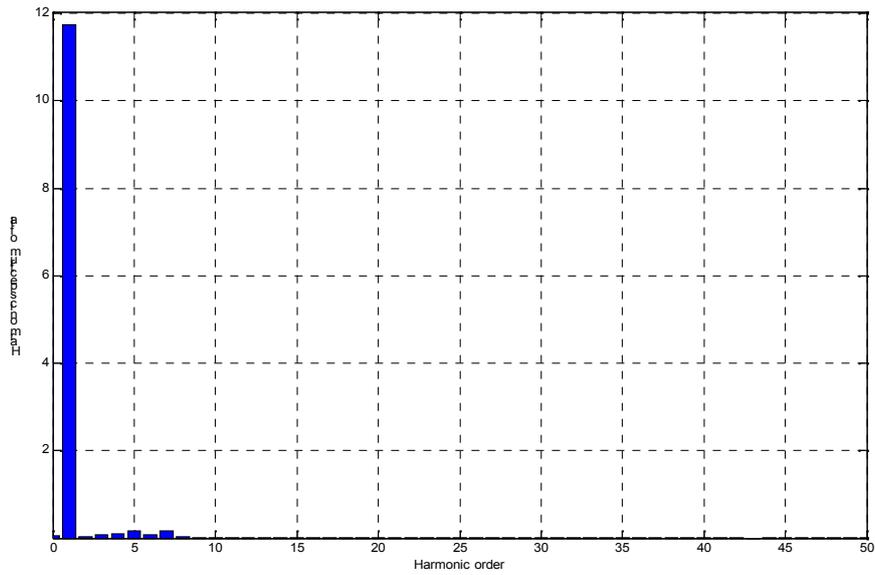
Fig.7.2. Total harmonic Distortion of Input Current of DPC
