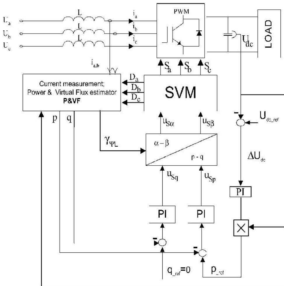
Fig. 4.1 Block scheme of Direct Power Control
