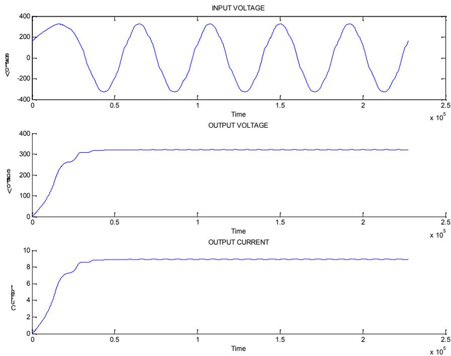
Fig. 6.5 (a) Waveforms of i) Input Voltage ii) Output Voltage iii) Output Current
