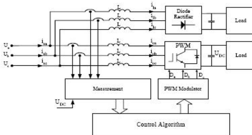
Fig 5.1. Block scheme of PWM Rectifier with active filtering function
