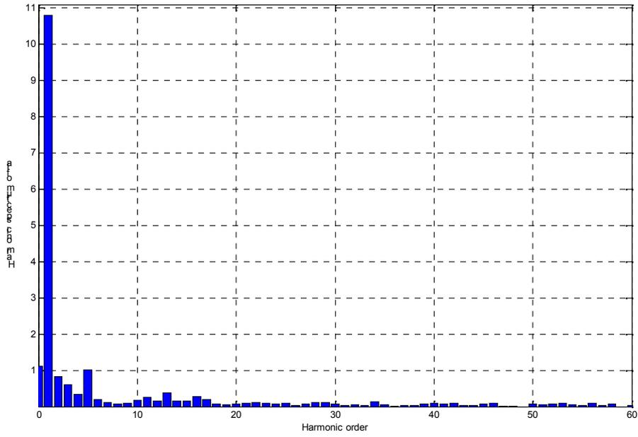
Fig.7.1. Total harmonic Distortion of Input Current of VOC
