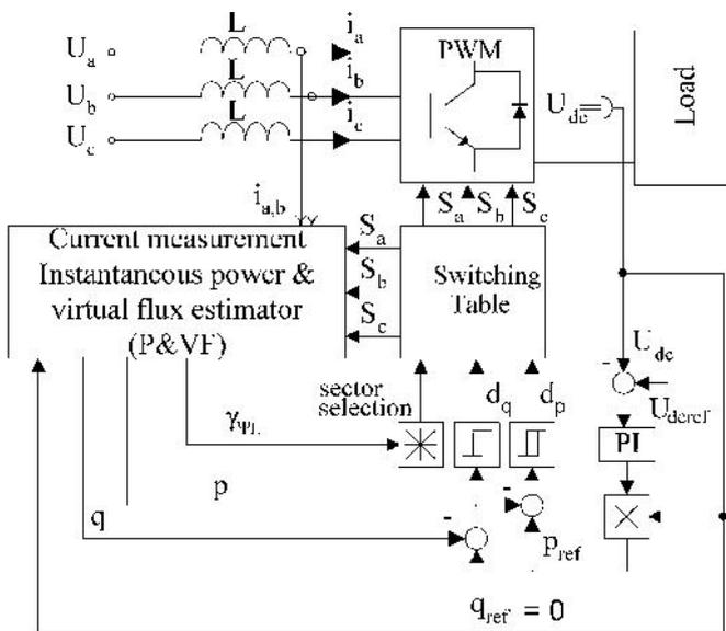
Fig.4.3. Block scheme of VF-DPC.
