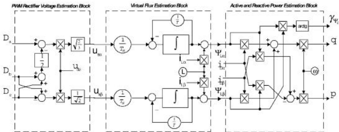
Fig. 4.4. (a) Block scheme of DPC-SVM. (b) Block scheme of DPC-SVM estimators (P&VF).
