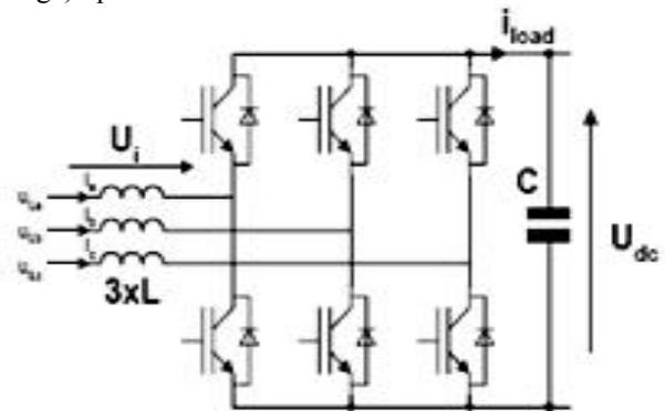
Fig. 1.4 (a) Boost topology of PWM rectifier
