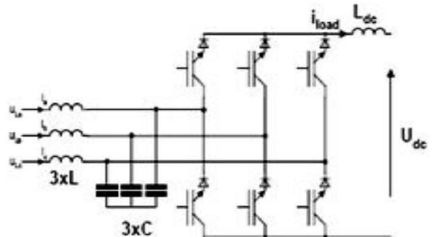
Fig. 1.4 b) Buck topology of PWM rectifier
