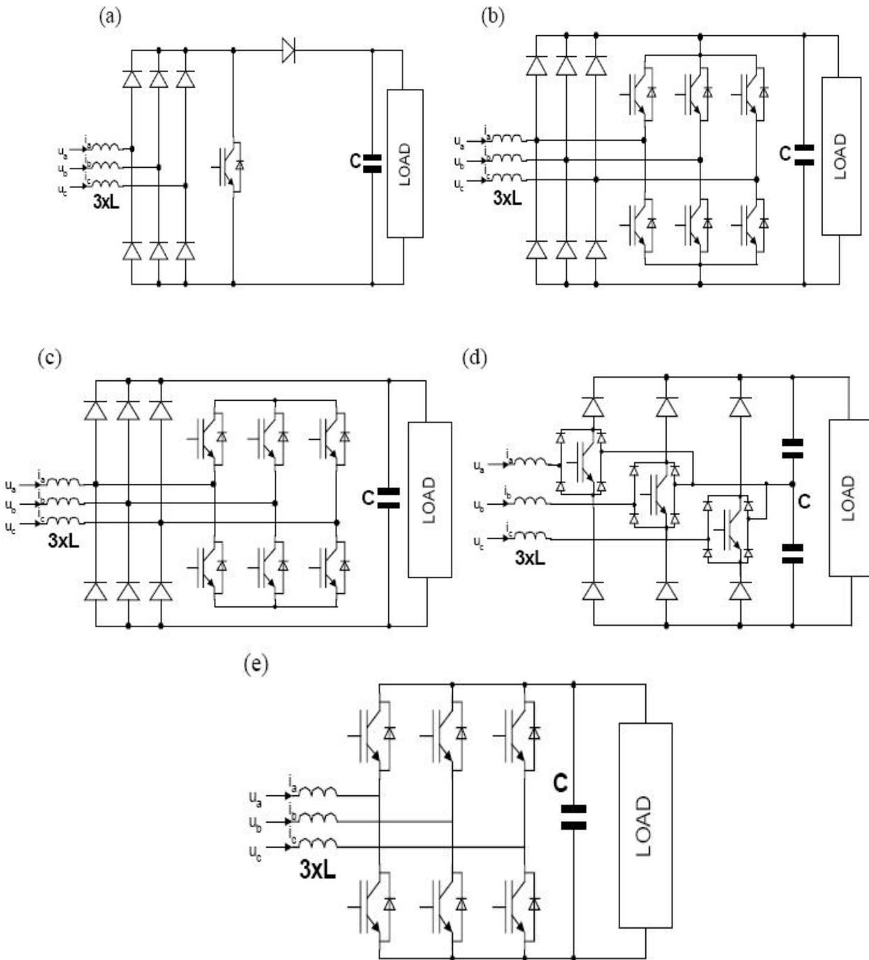
Fig.2.3 Basic topologies of switch-mode three-phase rectifiers: a) Simple boost-type converter; b) Diode rectifier with PWM regenerative braking rectifier; c) Diode rectifier with PWM active filtering rectifier; d) Vienna rectifier (3. level converter); e) PWM reversible rectifier (2 Level converter)
