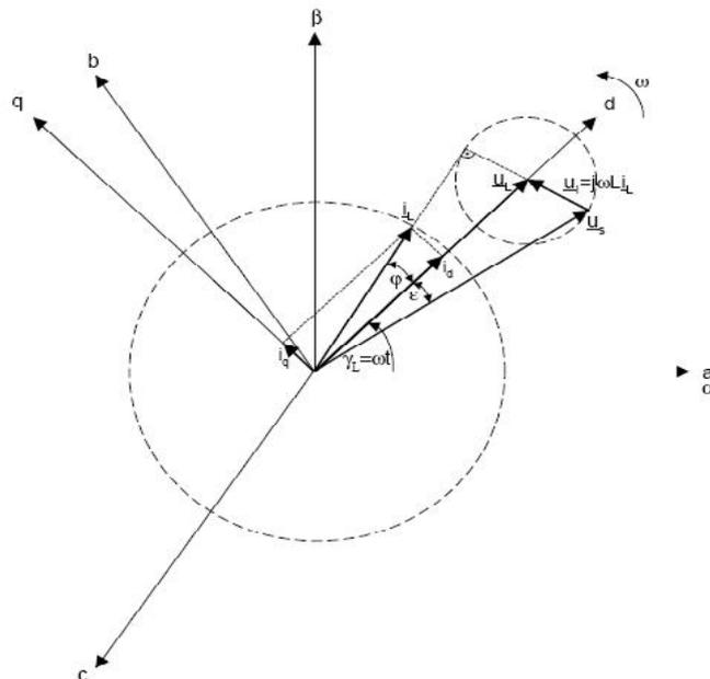
Fig. 2.9 Relationship between vectors in PWM Rectifier
