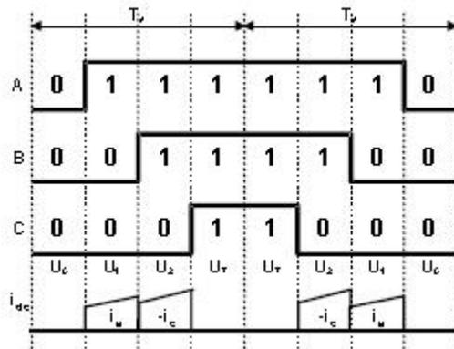
Fig. 2.14 PWM signals and DC link current in sector I
