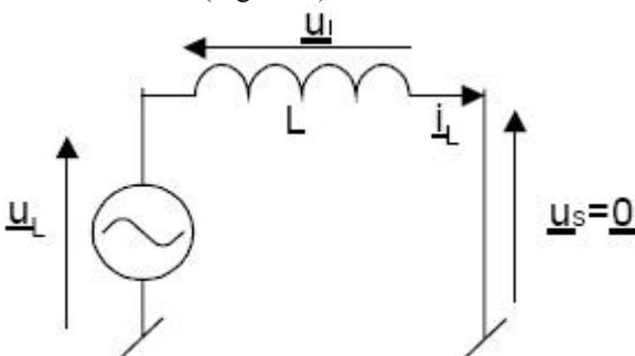
Fig. 2.16. PWM rectifier circuit when the zero voltage vector is applied.
