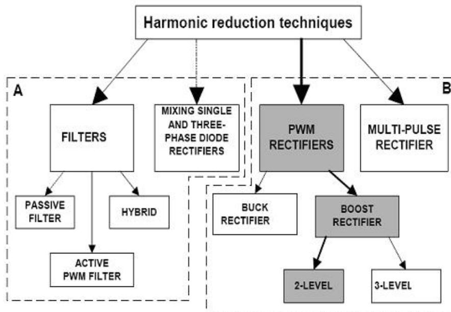
Fig. 1.1 Most popular three-phase harmonic reduction techniques of current
