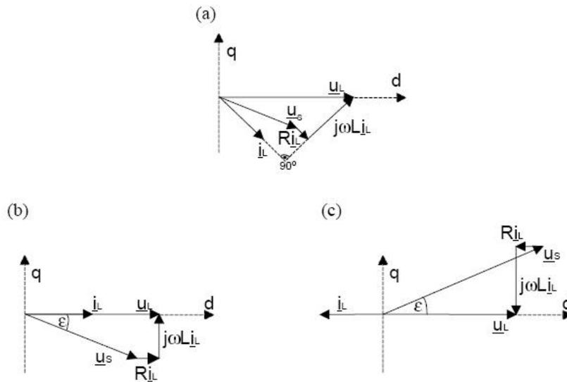
Fig. 2.7 (a) General Phasor diagram of the PWM rectifier
