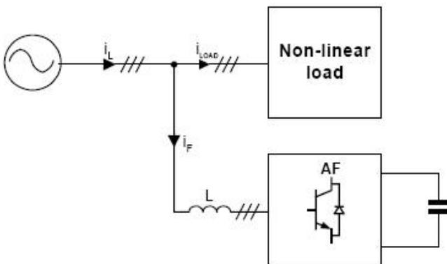
Fig. 1.2 Three-phase shunt Active filter
