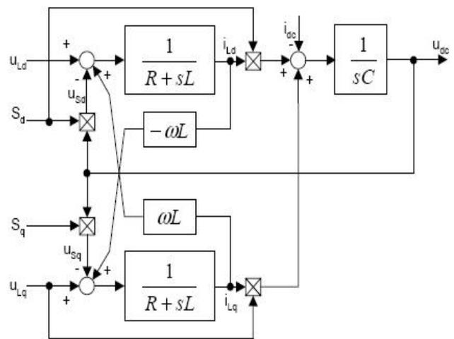
Fig. 2.12 Block diagram of voltage source PWM rectifier in synchronous  $d$ - $q$  coordinates
