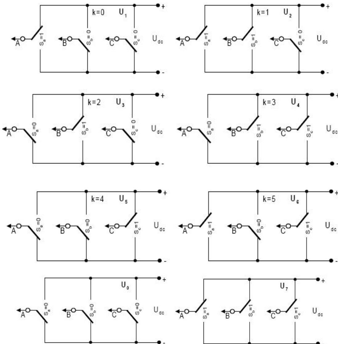
Fig. 2.8 Switching states of PWM bridge converter
