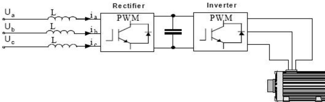
Fig. 2.4 AC/DC/AC converter
