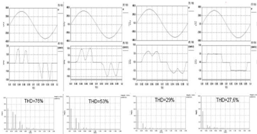
Fig. 2.2 Simulation results of diode rectifier at different input inductance (from 0 to infinity)
