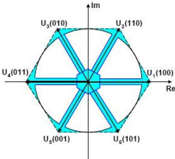
Fig. 2.15. Voltage vector area requiring the adjustment of PWM signals, when a reference voltage passes one of possible six active vectors and in case of low modulation index and over modulation
