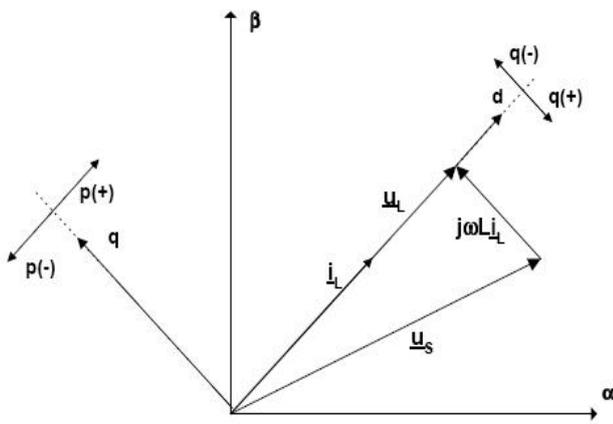
Fig. 2.13 Power flow in bi-directional AC/DC converter as dependency of *iL* direction.
