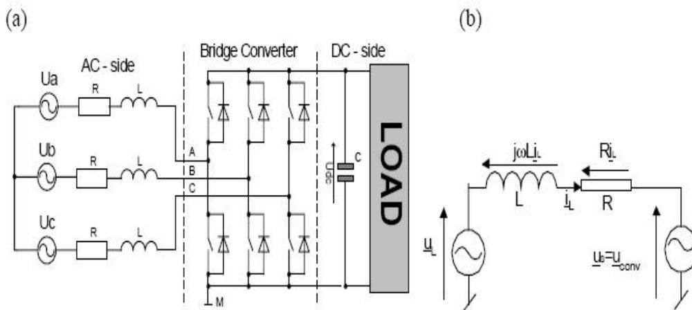
Fig. 2.6 (a) Three-phase PWM rectifier for bi-directional power flow.
