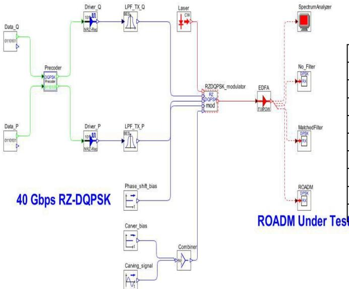
Fig. 2 Schematic of reconfigurable optical add drop multiplexer
