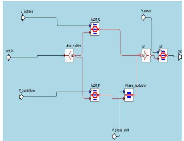
Fig. 3 a RZ-DQPSK modulator schematic
