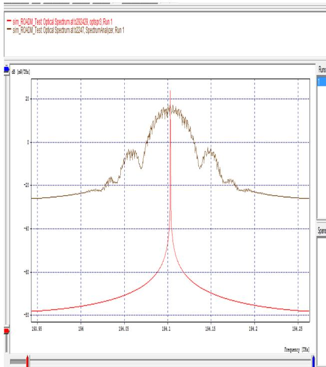
Fig. 8 optical spectrum at input and output of ROADM SYSTEM
