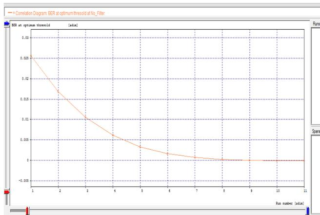
Fig.4 BER versus OSNR at optimal threshold at no filter
