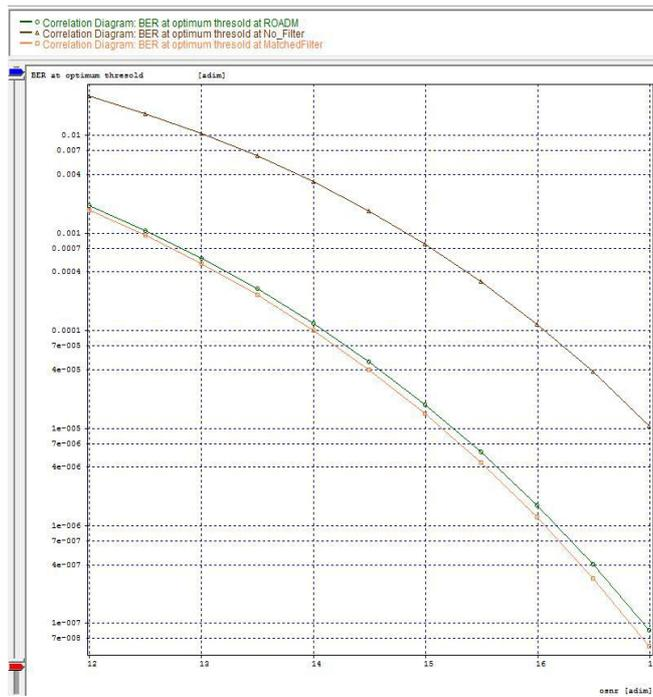
Fig. 7 BER versus OSNR plot for the ROADM under test as compared to matched filter and no filter at the receiver.
