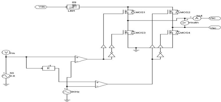
Fig 10: Inverter sub-circuit used in Simulation
