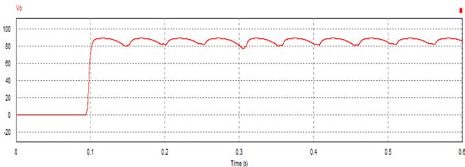
Fig 12 : Output of Rectifier stage
