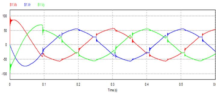
Fig11:Output of AC Synchronous Generator at 12m/s Wind-speed
