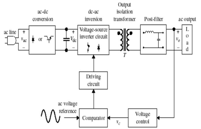
Fig 8: Block diagram of inverter stage
