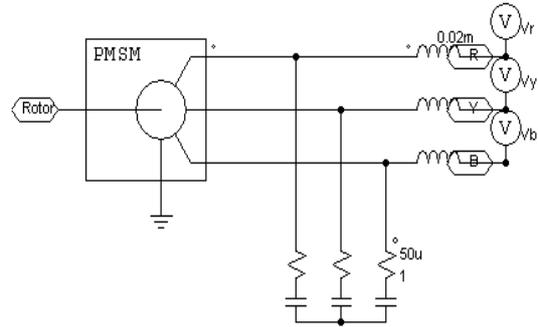
Fig 2: The Generator sub-circuit
