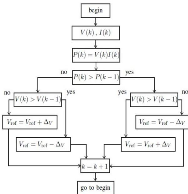
Fig 4: Flowchart of Perturb and Observe method
