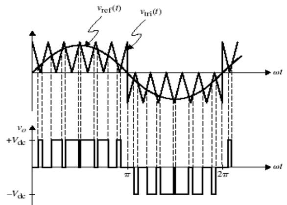
Fig 9: Typical Waveform for Sinusoidal Pulse Width Modulation Technique
