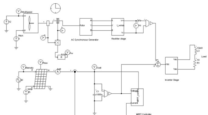
Fig 1: Block diagram of Wind solar hybrid system
