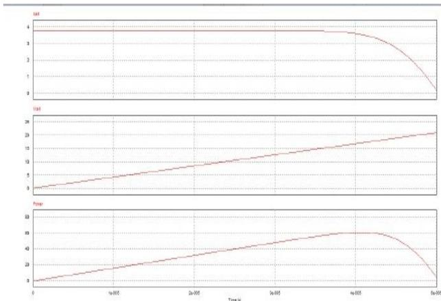
Fig 7: P-V characteristics of solar cell
