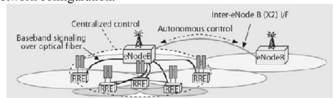
Fig. 1. CoMP Network configuration
