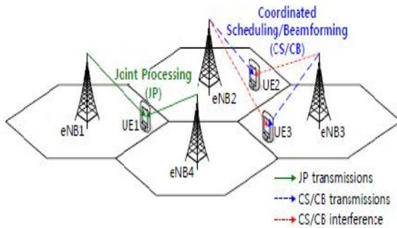
Fig. 2. CoMP architecture for CS/CB and JP transmissions.
