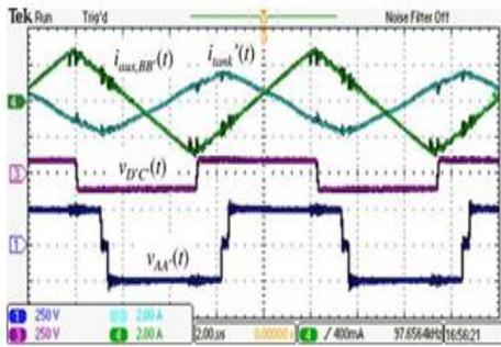
Fig. 15. Experimental waveforms for full ZVS operation with the proposed technique,  $P_{test} = 110\text{ W}$ ; voltage scale: 250 V/div; current scale: 2 A/div; time scale: 2 μs/div
