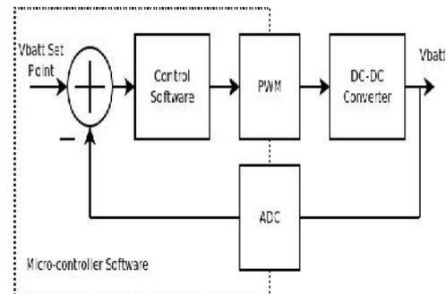
Figure: 1 block diagram of dc/dc converter
