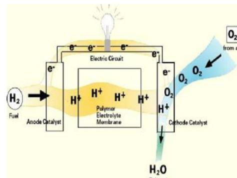
Encouraged by the catalyst, the hydrogen atom splits into a proton and an electron, which takes different paths to the cathode, the proton passes through the electrolyte, the electrons create a separate current that can be utilized before they return to the cathode, to be reunited with the hydrogen and oxygen in a molecule of water
