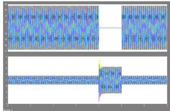
generating stations and the same power During Abnormal conditions with the NSFCL the current is limiting from a 400 AMPS to 40AMPS i.e it can limit the current 100:10 ratio is shown in a below waveform(D)
