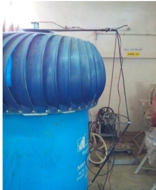
Figure 5(a) new wind solar driven natural turbine ventilator
