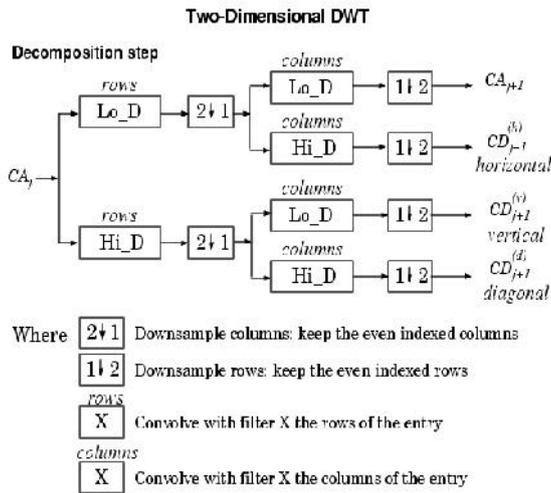
Fig 2: Decomposition Steps in 2-D DWT
