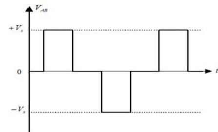
Output waveform of Full bridge Inverter
