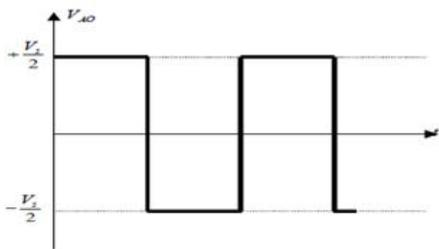
waveform of Half Bridge Inverter
