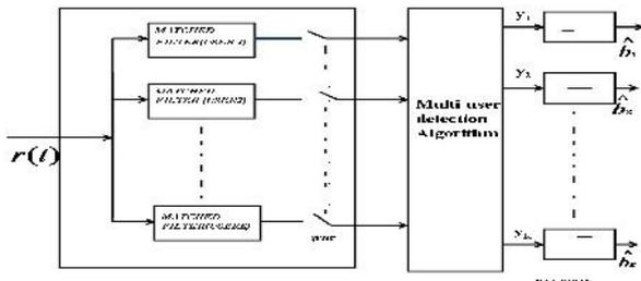
Fig.1: A typical multi-user detector
