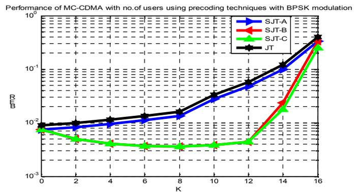
Fig. 6: BER versus  $K$  performance of precoding techniques of  $P = 3$  for  $\text{SNR} = 7 \text{ dB}$ ;  $L = 16$ ; orthogonal codes; BPSK modulation
