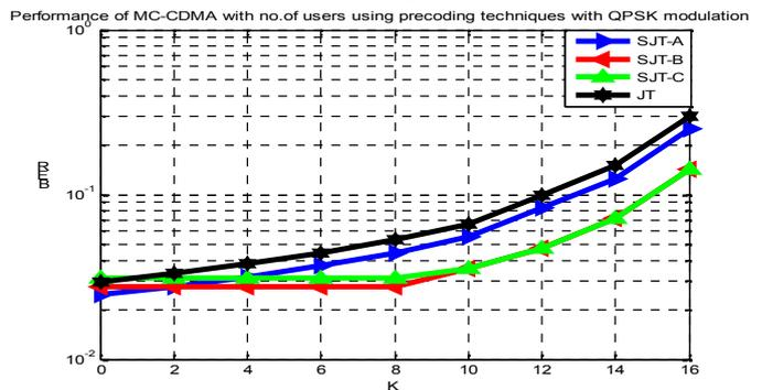
Fig. 7: BER versus  $K$  performance of precoding techniques of  $P = 3$  for  $\text{SNR} = 7 \text{ dB}$ ;  $L = 16$ ; orthogonal codes; QPSK modulation
