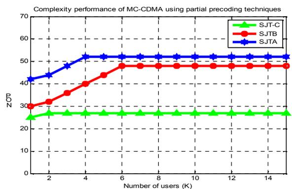
Fig. 9: Decorrelating complexity of the three proposed SJT techniques for  $L = 16$ ,  $P = 11$ , BPSK modulation, and  $\text{SNR} = 7 \text{ dB}$
