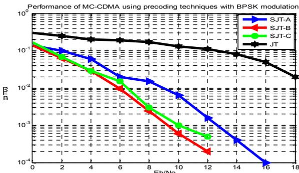
Fig. 3: BER versus SNR performance of the three proposed SJT precoding methods in a Rayleigh fading channel of  $P = 3$  paths for  $K = 5$ ;  $L = 16$ ; with BPSK modulation.
