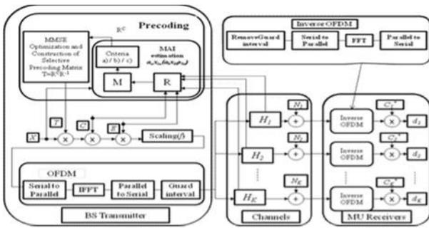
Fig.2: The proposed selective pre-coding in the MC-CDMA downlink
