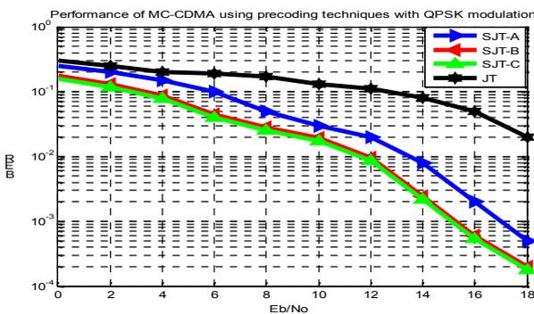
Fig. 4: BER versus SNR performance of the three proposed SJT precoding methods in a Rayleigh fading channel of  $P = 3$  paths for  $K = 5$ ;  $L = 16$ ; QPSK modulation.
