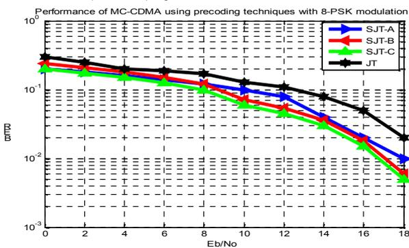
Fig. 5: BER versus SNR performance of the three proposed SJT precoding methods in a Rayleigh fading channel of  $P = 3$  paths for  $K = 5$ ;  $L = 16$ ; 8-PSK modulation.
