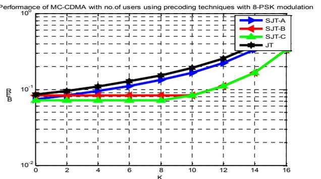
Fig. 8: BER versus  $K$  performance of conventional JT and SJT in a Rayleigh channel of  $P = 3$  for  $\text{SNR} = 7 \text{ dB}$ ;  $L = 16$ ; 8-PSK modulation
