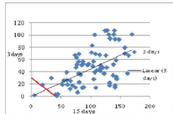
**Fig.5.** cumulative rainfall plot of 3 vs. 15 days rainfall prior to landslide event
