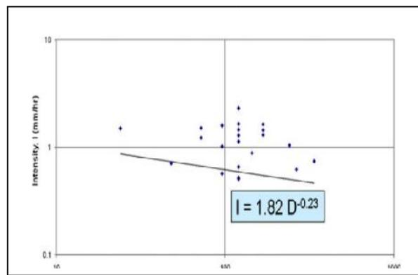
**Fig.4.** Rainfall intensity-duration (ID) threshold based on estimation of daily rainfall data for the initiations of landslide in Chamoli- Joshimath [7]
