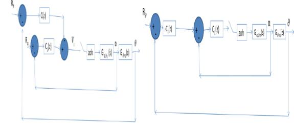
Fig (6) Block diagram of RIP
