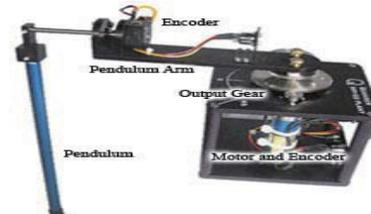
Fig (1) Rotary inverted pendulum model SRV-2.
