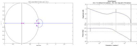
Fig (11) Root locus diagram of RIP final system
