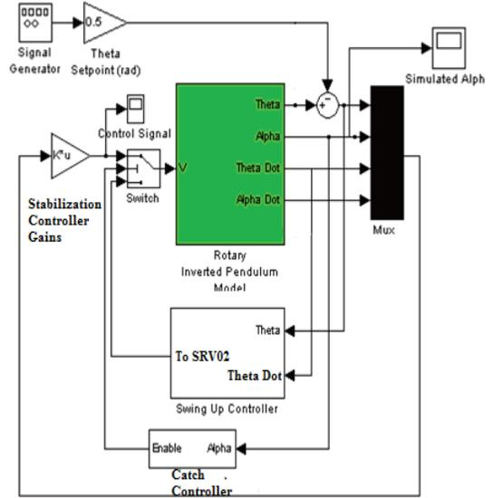
Fig (3) Block diagram Controller for rotary inverted pendulum model (MATLAB Simulink).
