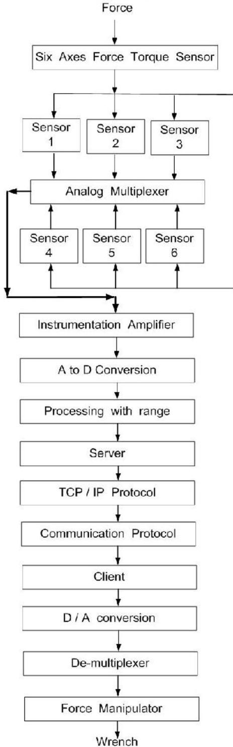
Fig. 4 Flow chart of the implemented software
