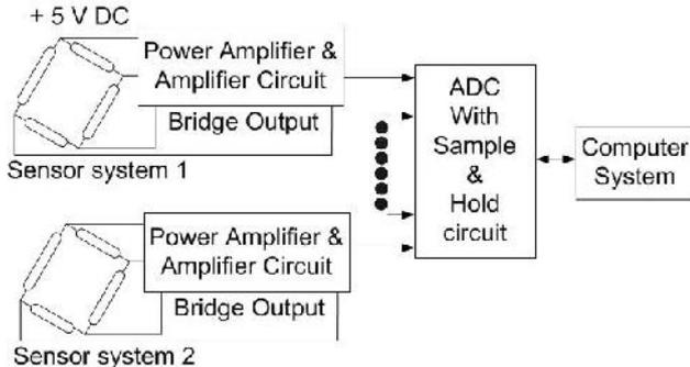
Fig. 2 Interface details of the sensing system
