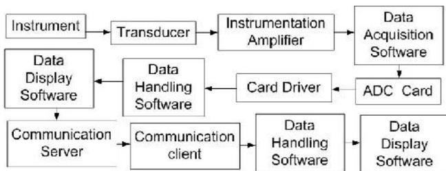
Fig. 1 Block diagram of the designed system
