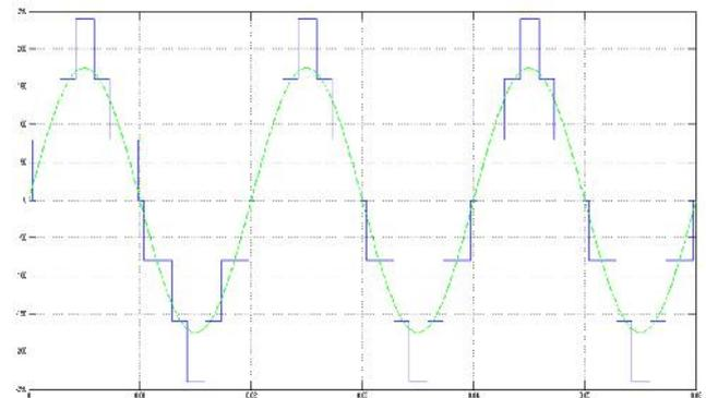
Fig3: Final output waveform from the inverter
