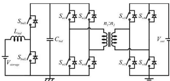
Fig. 1.c. DAB including a bidirectional converter
