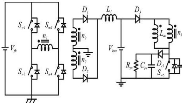
Fig. 3. Proposed converter with dissipative passive clamping circuit
