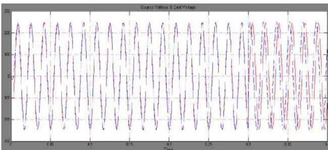
Fig.11 Synchronization of Source Voltage & Grid Voltage
