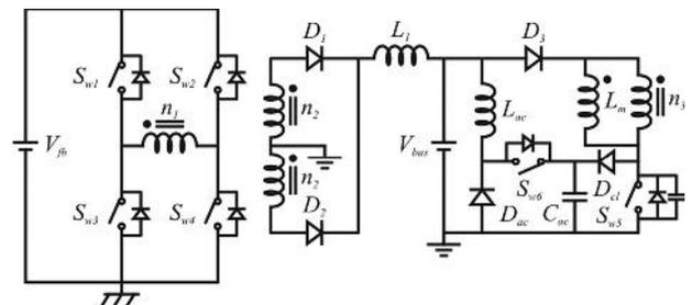
Fig. 4. Proposed converter with regenerative active clamping circuit
