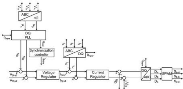
Fig.6. Constant Voltage Current Controller
