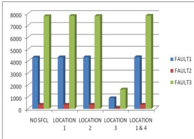
Figure 6 Comparison of the reduction in wind farm fault current magnitude in Three Phase to Ground Fault Case.
