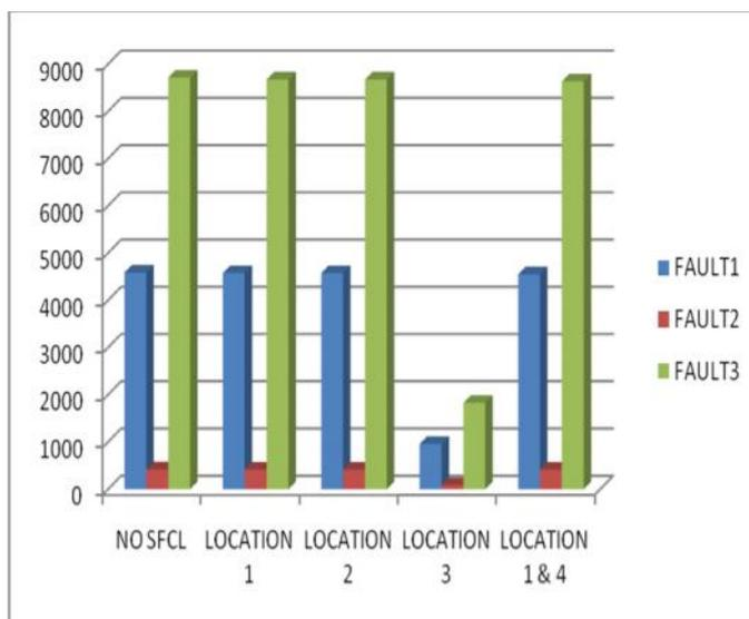
Figure 8 Comparison of the reduction in wind farm fault current magnitude Phase to Phase Fault Case.
