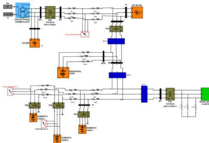
Figure 1 Power system model designed in Simulink. Fault (Red) and SFCL (Blue) locations are indicated in the diagram.
