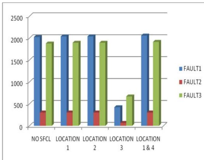
Figure 7 Comparison of the reduction in wind farm fault current magnitude Single Phase to Ground Fault Case.
